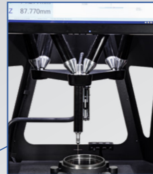
Robust design utilising linear motors and mechanical bearings.
