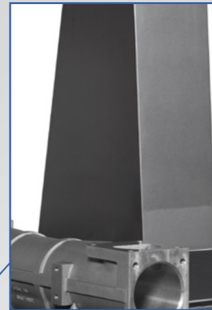
Redesigned right leg for improved stiffness and accuracy.
